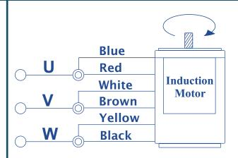
For the Voltage 230 VAC, 3-Phase Supply, Wires are connected as shown in the fig. Short Blue & Red, Black & Yellow, and White& Red as per the fig. Shown.
