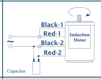
Black Wires are for Starting purpose and Red wires for the Running purpose, as shown in fig.,
