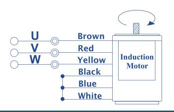
For the Voltage 415 VAC, 3-Phase Supply, Wires are connected as shown in the fig. Short Blue, Black and White and then insulate it carefully.
