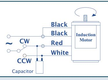
Short the Black wires and connect as shown in fig., To rotate the motor in Clockwise direction.
